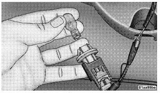
3. Replace the bulb and reinstall the socket into the housing by locking it in place with a twist.
